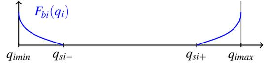
Fig. 4: Repulsive field outside the safe interval.
