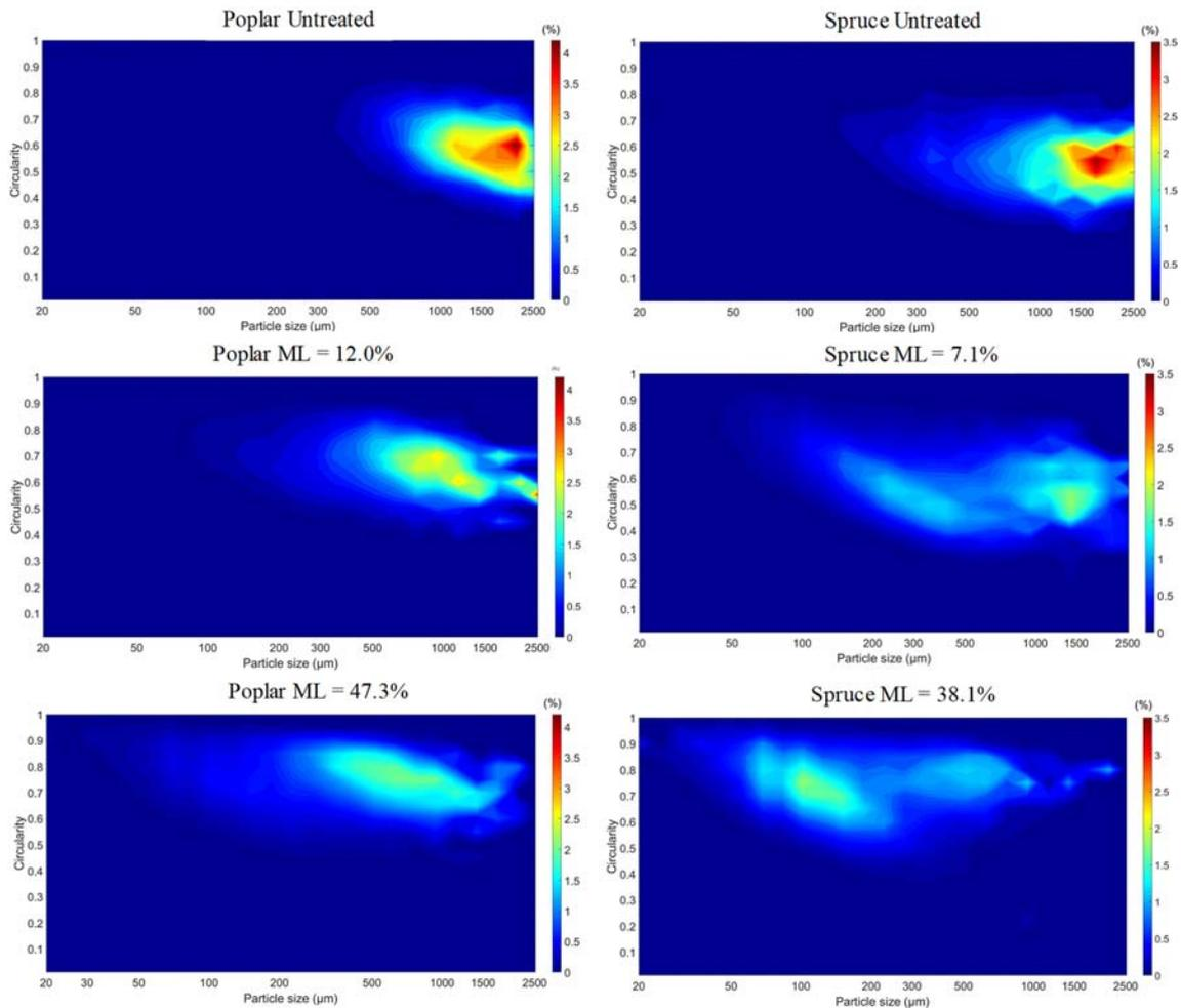
*Figure 2. Influence of torrefaction intensity on circularity and size distributions for spruce and poplar powders. The colour scale indicates the volume fraction of each size and shape range and varies between the same values regardless of the torrefaction intensity for each species.*
