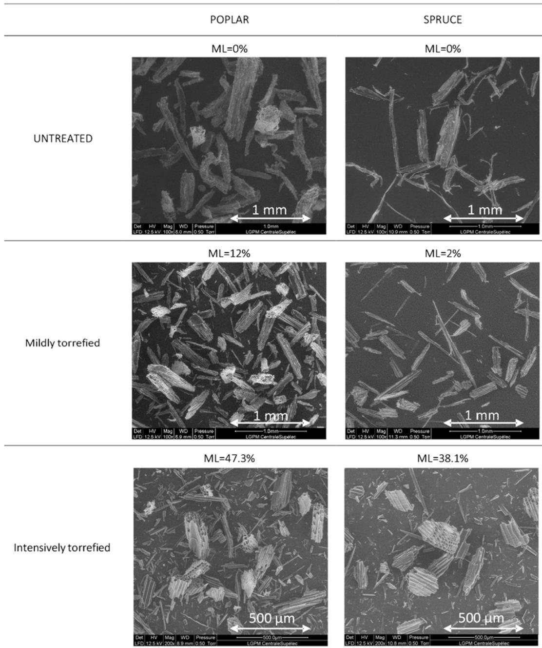
Figure 8. Scanning Electronic Microscopic images for untreated and torrefied spruce and poplar powders.
