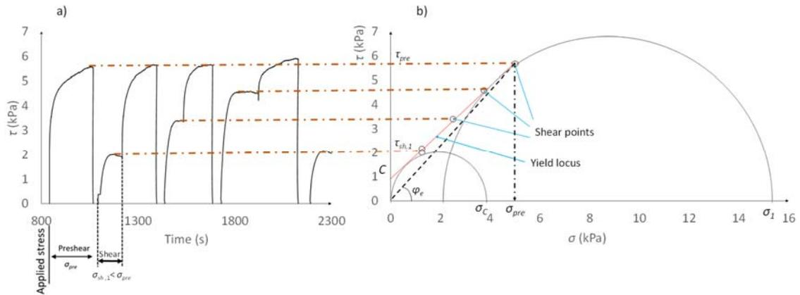
Figure 1. Flow properties determination (Untreated poplar sample,  $\sigma_{pre} = 5$  kPa). a). Experimental course of shear stress; b) yield locus construction and Mohr stress circles defining unconfined yield strength and consolidation stress.
