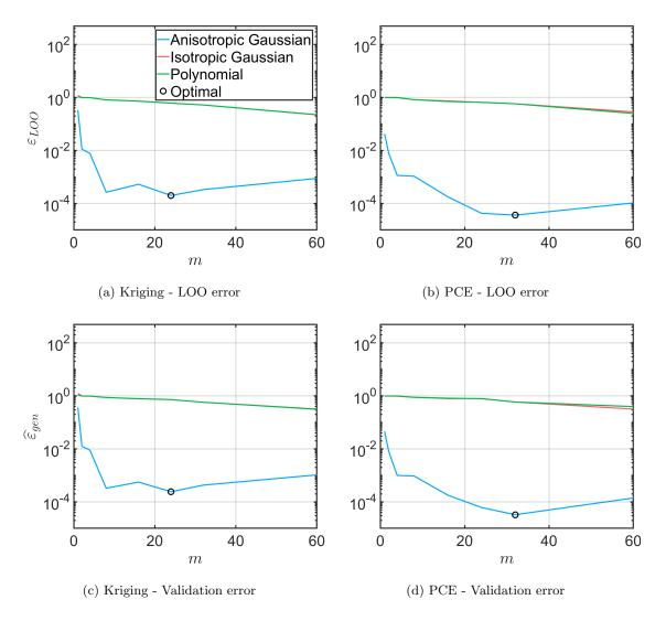
Figure 5: Electrical resistor networks: error estimates of the DRSM surrogate as a function of the reduced dimension. Kernel PCA is used with anisotropic (resp. isotropic) Gaussian as well as polynomial kernels.
