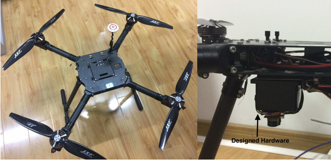
Fig. 5: A quadrotor is used for validation of the attitude estimation system involving MARG sensors and a monocular camera.
