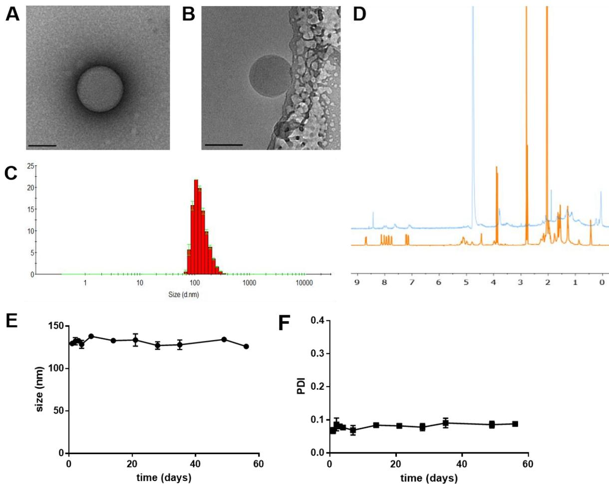
**Figure 2.** Characterization of **nano-rac-2**. TEM (A) and cryo-TEM image (scale 100 nm) (B) DLS size distribution showing (C), overlay of  $^1\text{H-NMR}$  of **2** (orange) and **nano-rac-2** (blue) in deuterated acetone and water, respectively (D), and size (E) and PDI stability (F).
