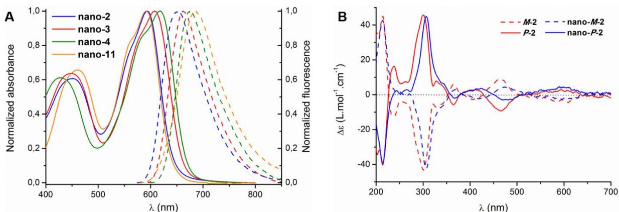
**Figure 4.** Normalized absorption (plain lines) and fluorescence (dashed lines) spectra of racemic NAs in water (A) and UV-vis electronic circular dichroism spectra of *M-2* (dashed lines) and *P-2* (plain lines) single molecules (acetonitrile, red) and NAs ( $\text{H}_2\text{O}$ , blue) (B).
