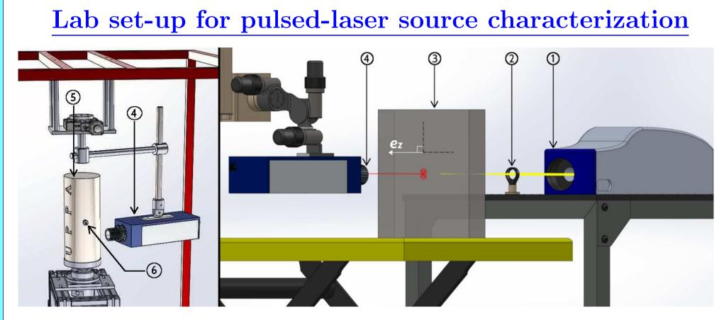
Two different experimental tools were mounted to investigate in Cartesian coordinates or in cylinder coordinates. ①: Q-Switched laser generator; ②: convergent lens; (3): Aluminium cuboid samples of various thickness (10, 50, 100 mm),  $V_p \approx 6350$  m/s,  $V_s \approx V_p/2$ ; 4: single point Laser Doppler Vibrometer (LDV); (5) core sample; (6) piezoelectric source.
