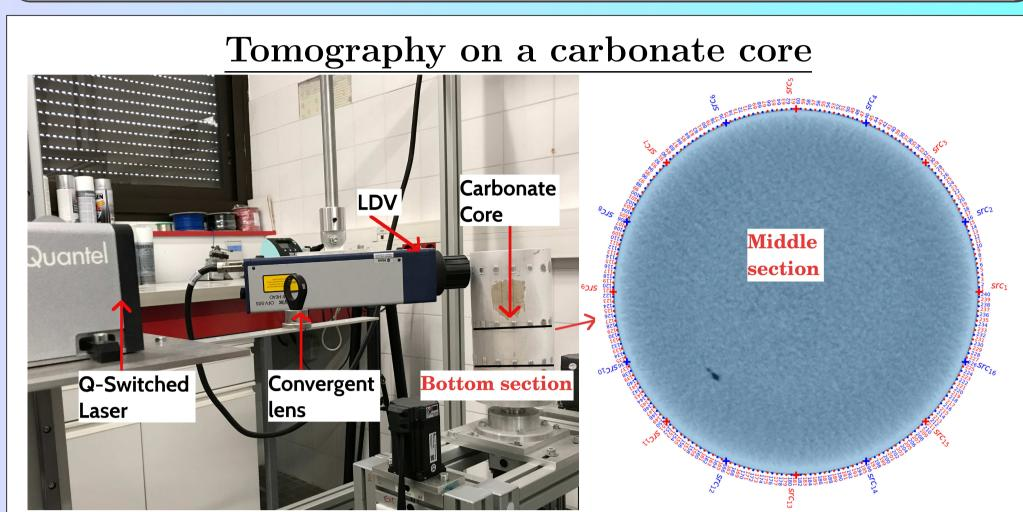
Application of the pulsed-laser ablation source on a carbonate core ( $\Phi \approx 120mm$ ). We used the point-source point-receiver setup. 16 sources (aluminum flakes) are uniformly distributed along the circumference of each normal section. Each source covers 300° (101 receivers @ 3°) in a symmetric
