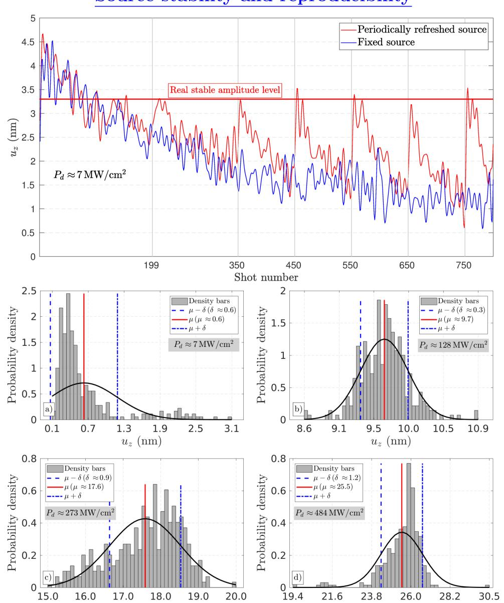
Distribution of first arrival seismic wave amplitudes  $u_z$  measured by LDV at the epicenter of the 10 mm thick aluminum block.  $P_d$  denotes the incident power
