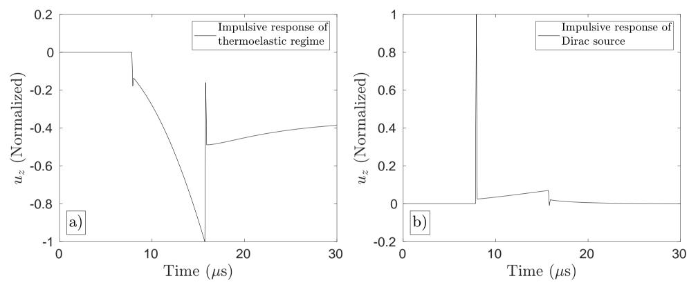
a): laser-generated seismic source under thermoelastic regime with displacements computed by combining the wave equation and the thermoelastic equations [2, 3, 5]. b): laser-generated seismic source under ablation regime which is modelled as a point-source [1, 2].
