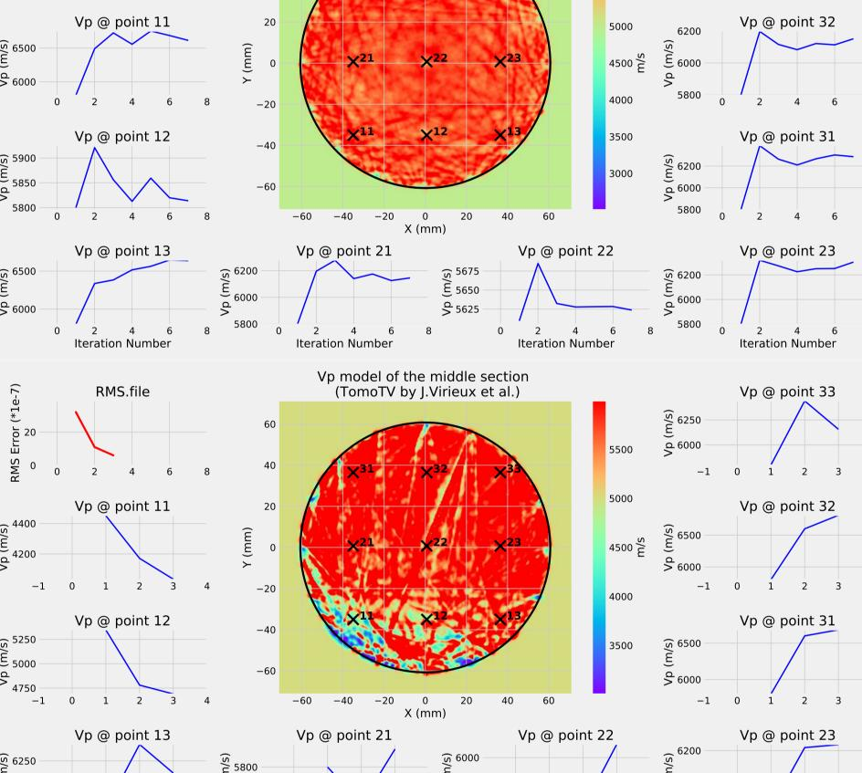
Considerable diffractions caused by the cavity disturbs heavily the first arrival time  $(2^{nd} \text{ Tomo})$ The first break based inversion algorithm doesn't take into account this complicated phenomenon. leading to noisy, unstable and hardly convergent results.
