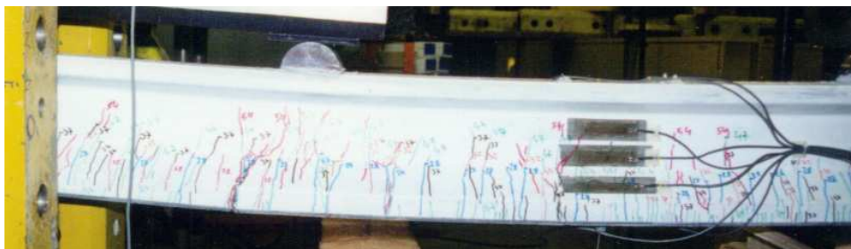
Figure 1: Evidence of ductility, test for approval of UHPFRC beams in view of their application in the renovation of thermal exchange devices in Cattenom plant cooling tower [3]
