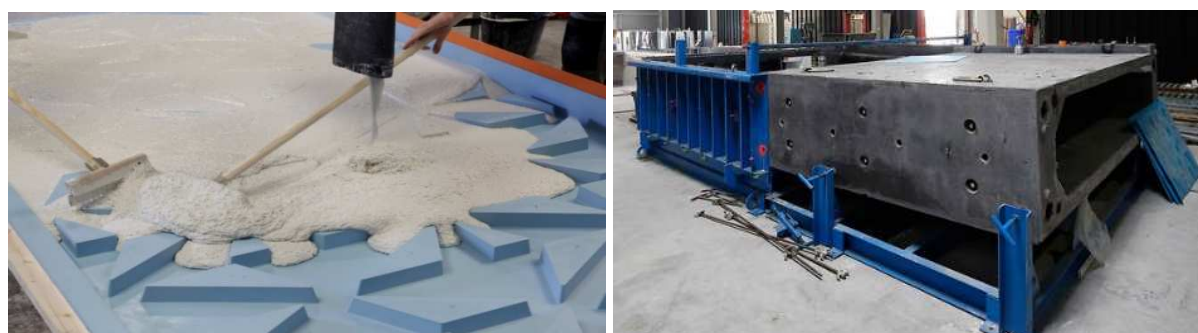
Figure 17: Typical form solutions for UHPFRC elements. Left) supply material for the mould of a net panel with numerous inclusions [36]. Right) Match-casting of thin walled segments to be assembled by post-tension [22].
