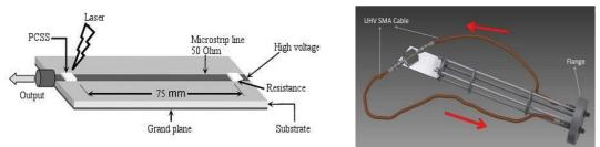
Figure 1. Nonlinear loaded microstrip generator (in left) and the transmitting system (in right).
