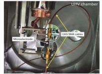
**Figure 4.** Photography of atom probe analysis chamber with proposed microstrip TL (microelectrode).
