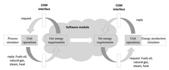
Figure 4. The cornerstone of the proposed framework: data exchange between process and energy simulators via COM interface.
