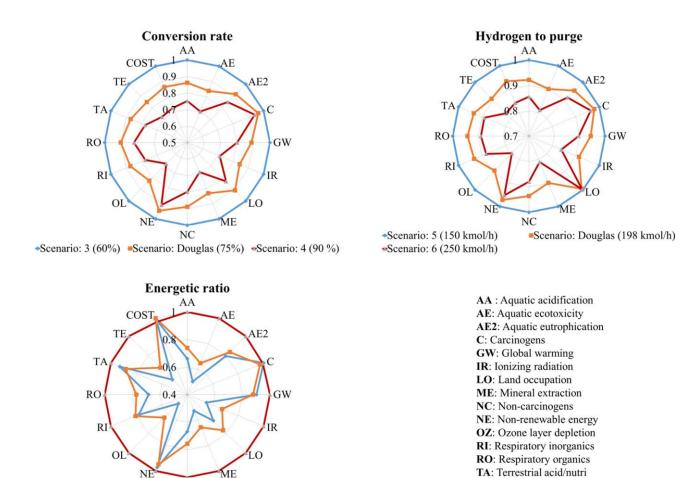
**Figure 13.** Classification of the environmental impact and cost criteria according to the variables conversion rate ( $C_{\text{rate}}$ ), hydro gen flowrate ( $F_{\text{H2}}$ ), and energetic ratio ( $R_{\text{Fuel}}$ ) (mid points).
