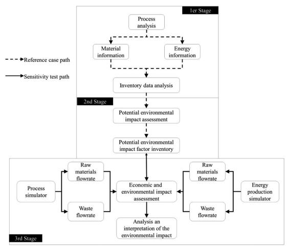
Figure 1. Overview of the proposed approach for eco efficient process design through the integration of the LCA and process simulation.
