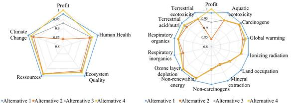
Figure 19. Comparison of profit and environmental criteria of the four process alternatives.
