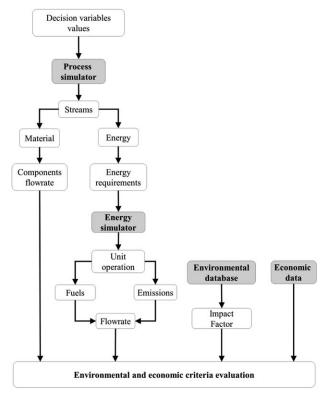
**Figure 2.** Exchange and retrieval of data between the simu lation models and impact factor database for eco efficient process design.
