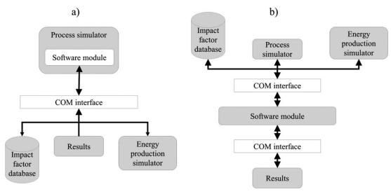
**Figure 3.** Possible framework architectures: (a) embedded in process simulator with a programming interface and (b) with an independent platform with a COM interface.
