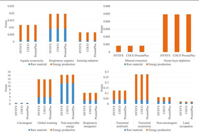
**Figure 6.** Contribution to mid point categories of the raw materials and the production of the energy requirements of the process (normalization).
