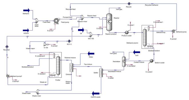
**Figure 18.** Flowsheet of biodiesel production process.
