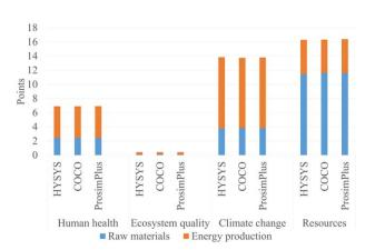
**Figure 7.** Contribution to end point categories of the raw materials and the production of the energy requirements of the process (normalization).
