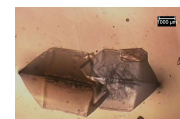
Figure 4 Epitaxy of \text{NaClO}_3 showing two opposite handedness obtained by evaporation of solvent at room temperature in presence of \text{Na}_2\text{S}_2\text{O}_6 .
