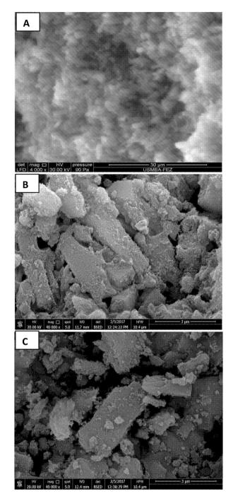
**Figure 3.** SEM photographs of the parent ZSM-5 (A), Fe-ZSM-5 (B), and Cu-ZSM5 (C).
