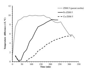
**Figure 6.** Comparison of temperature difference ( $\Delta T$ , °C) between the inlet and outlet of the adsorbent bed reactor during ozone decomposition by Fe-ZSM-5, Cu-ZSM-5, and parent zeolite ZSM-5.
