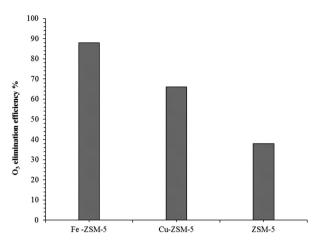
Figure 5. Ozone removal efficiency of ZSM-5 (parent zeolite), Fe- ZSM-5, and Cu-ZSM-5 samples.
