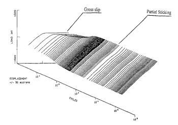
Fig. 3 Friction log for a 7075 alloy test. Fn = 100 daN;  $\delta = +/-35 \mu m$  frequency = 5 Hz;  $\sigma_0 = 230$  MPa; number of cycles = 3.10<sup>5</sup>.
