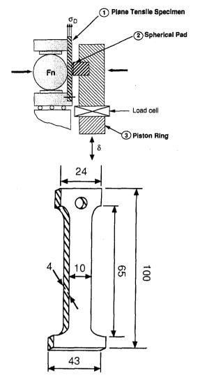
Fig. 2 Fretting fatigue apparatus and plane tensile specimen dimensions (in millimeters)
