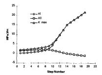
Fig. 7(a) Variation of KI, KII and K $\sigma$  max for crack 1, during a whole cycle
