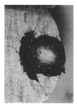
Fig. 4(a) View of the surface contact. "eye-shape" of the cracks
