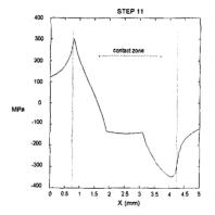
Fig. 6 Variation of σxx stress field at the surface of the slab for 4 steps of the 11 step-cycle for a 7075 alloy. (See experimental conditions Table 2.)
