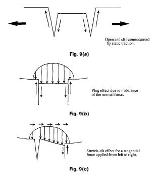
Fig. 9 Mechanisms induced by external loadings;(a) Slip zones induced by static traction; (b) Plug effect caused by normal forces; (c) Stretchtilt effect caused by tangential force.
