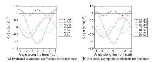
Figure 9. Inclined (45°) penny shaped crack under remote tension. Numerical results for a graded mesh (T-stress is normalized by  $\sigma$ ). An order one finite elements discretization is used along the front for the three modes. (a) Evaluated asymptotic coefficients for coarse mesh. (b) Evaluated asymptotic coefficients for fine mesh.
