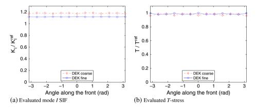
Figure 5. Penny shaped crack under remote tension. Numerical results of the comparison between a coarse mesh and a fine mesh,  $ds \simeq 2$  finite elements of the coarse mesh, and four finite elements of the fine mesh. (a) Evaluated mode *I* SIF. (b) Evaluated *T*-stress.
