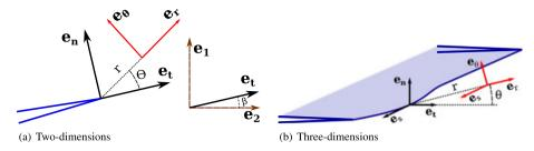
Figure 1. Local coordinate system around the crack tip. (a) Two-dimensions. (b) Three-dimensions.
