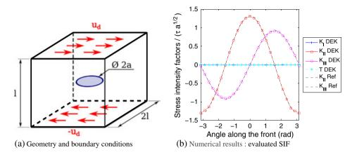
Figure 7. Penny shaped crack under remote shear. (a) Geometry and boundary conditions. (b) Numerical results: evaluated SIF.
