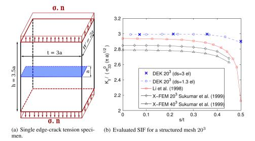
Figure 13. Single edge-crack tension specimen, with the monogrid mesh used in Sukumar *et al.* [38]. (a) Single edge-crack tension specimen. (b) Evaluated SIF for a structured mesh 20<sup>3</sup>.
