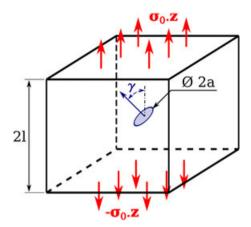
Figure 8. Geometry and boundary conditions of the inclined (45°) penny shaped crack under remote tension.
