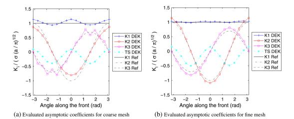
Figure 10. Inclined (45°) penny shaped crack under remote tension. Numerical results for a graded mesh (*T*-stress is normalized by  $\sigma$ ). The direct extraction is based on Equation (30) where  $\varphi_s(s)$  are order one finite elements shape functions and  $\varphi'_s(s)$  are order zero. (a) Evaluated asymptotic coefficients for coarse mesh. (b) Evaluated asymptotic coefficients for fine mesh.
