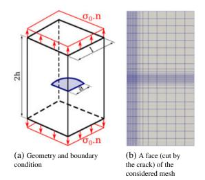
Figure 11. Corner edge cracked bar. (a) Geometry and boundary condition. (b) A face (cut by the crack) of the considered mesh.
