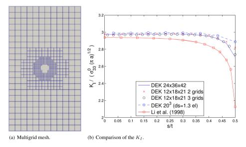
Figure 14. Single edge-crack tension specimen, with the localized multigrid method. (a) Multigrid mesh. (b) Comparison of the  $K_I$ .
