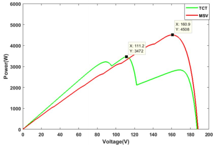
**Figure. 2. P-V characteristics of TCT and MSV for short wide pattern Pattern.**
