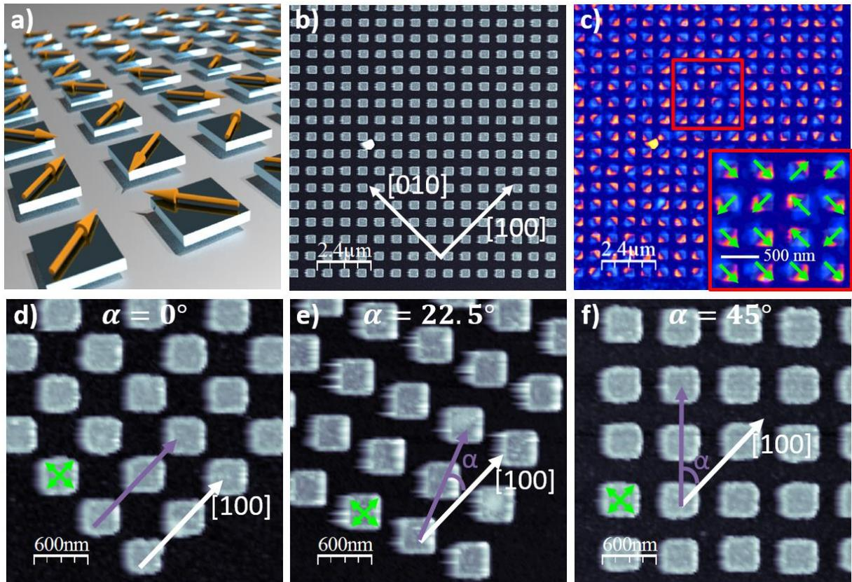
**Fig. 1 | Presentation of the system and geometry definition.** **a**, schematic diagram of the artificial spin system. **b**, Atomic Force Microscopy (AFM) image of a portion of the lattice. **c**, Corresponding Magnetic Force Microscopy (MFM) image. The zoom indicates the correspondence between the MFM contrast and the spin value. **d-f**, AFM images describing the three
