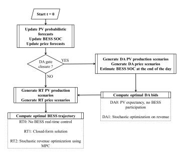
Fig. 1. Flowchart of the control algorithm
