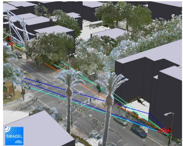
Figure 10 : Multipath prediction for a street-level backhaul link
