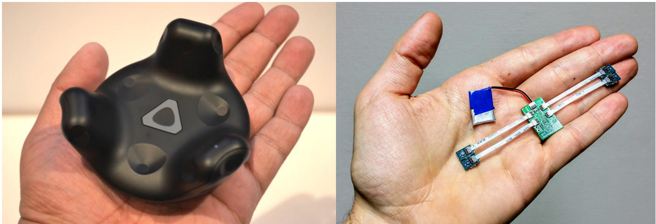
Figure 10: Size/weight comparison. Commercial tracker: 10 \times 10 \times 4.2 = 420\text{cm}^3 ; 85g. Hive Tracker: 2.5 \times 1.5 \times 1.1 = 4.13\text{cm}^3 ; 8g.
