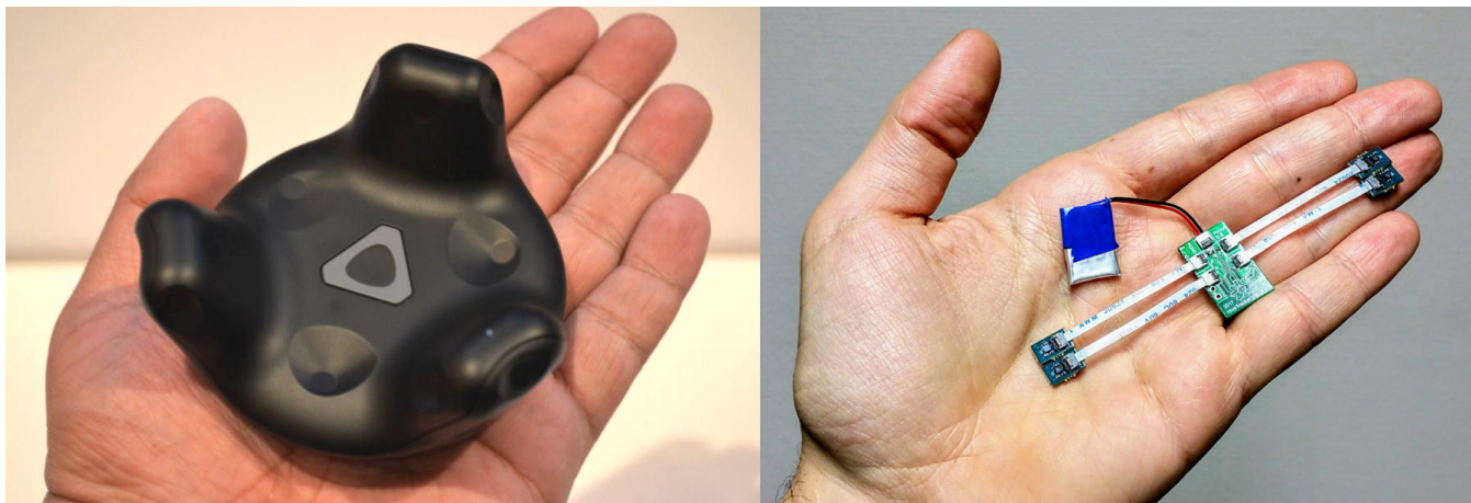
Figure 10: Size/weight comparison. Commercial tracker: 10 \times 10 \times 4.2 = 420\text{cm}^3 ; 85g. Hive Tracker: 2.5 \times 1.5 \times 1.1 = 4.13\text{cm}^3 ; 8g.
