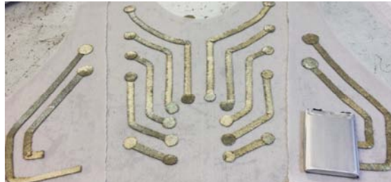
Figure 3 – Traces are added to fabric by layering heat bonding method
