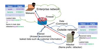
FIGURE 5: Information leakage attack through steganography-embedded Interest name.
