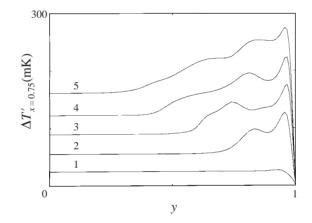
FIGURE 16. Temperature profiles at x = 0.75 for t' = 1.19 s (1), t' = 3.57 s (2), t' = 7.14 s (3), t' = 11.9 s (4) and t' = 23.8 s (5) for  $T'_i = T'_c + 15$  K and  $\rho'_i = \rho'_c + 125$  kg m<sup>-3</sup>.
