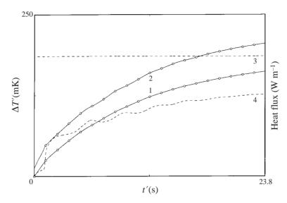
FIGURE 17. For  $T'_i = T'_c + 15$  K and  $\rho'_i = \rho'_c + 125$  kg m<sup>-3</sup>, temperature elevation versus time: bulk value (1) and mean value (2); dashed lines: heat fluxes injected by the thermistor (3) and lost at the upper wall (4).
