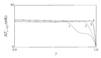
FIGURE 11. Temperature profiles around the cold boundary layer when the rising plume begins to strike the wall (at x = 0.5) for different times: t' = 0.76 s (curve 1), t' = 0.81 s (curve 2), t' = 0.86 s (curve 3), t' = 0.91 s (curve 4).
