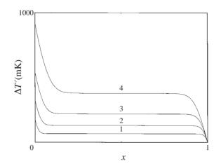
FIGURE 14. Temperature profiles in one dimension with P' = 74 W m<sup>-2</sup>, at t' = 4.76 s (1), t' = 11.9 s (2), t' = 23.8 s (3) and t' = 47.6 s (4).
