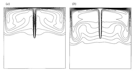
FIGURE 15. Thermal field at (a) t' = 7.14 s and (b) t' = 19 s for  $T'_{i} = T'_{c} + 15$  K and  $\rho'_{i} = \rho'_{c} + 125$  kg m<sup>-3</sup>.
