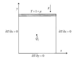
FIGURE 1. The centre-heated two-dimensional square cavity.
