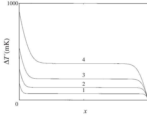
FIGURE 14. Temperature profiles in one dimension with  $P' = 74 \text{ W m}^{-2}$ , at  $t' = 4.76 \text{ s}$  (1),  $t' = 11.9 \text{ s}$  (2),  $t' = 23.8 \text{ s}$  (3) and  $t' = 47.6 \text{ s}$  (4).
