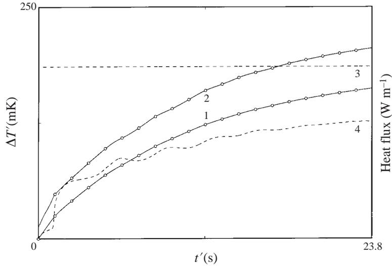
FIGURE 17. For  $T'_i = T'_c + 15 \text{ K}$  and  $\rho'_i = \rho'_c + 125 \text{ kg m}^{-3}$ , temperature elevation versus time: bulk value (1) and mean value (2); dashed lines: heat fluxes injected by the thermistor (3) and lost at the upper wall (4).
