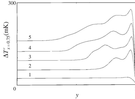
FIGURE 16. Temperature profiles at  $x = 0.75$  for  $t' = 1.19$  s (1),  $t' = 3.57$  s (2),  $t' = 7.14$  s (3),  $t' = 11.9$  s (4) and  $t' = 23.8$  s (5) for  $T'_i = T'_c + 15$  K and  $\rho'_i = \rho'_c + 125$  kg m $^{-3}$ .
