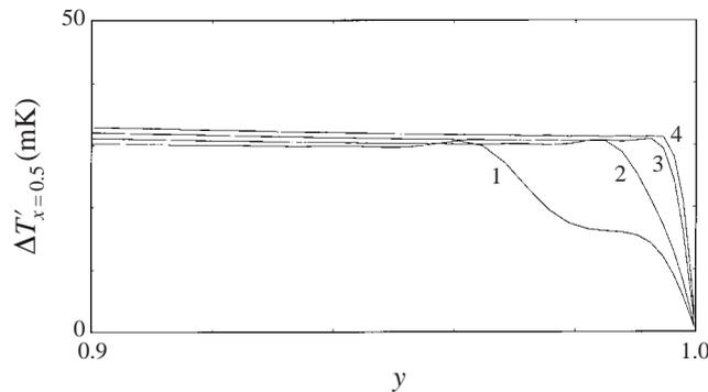
FIGURE 11. Temperature profiles around the cold boundary layer when the rising plume begins to strike the wall (at  $x = 0.5$ ) for different times:  $t' = 0.76$  s (curve 1),  $t' = 0.81$  s (curve 2),  $t' = 0.86$  s (curve 3),  $t' = 0.91$  s (curve 4).
