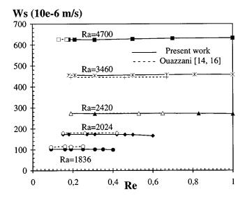
FIG. 11. Saturation amplitude of the vertical velocity component as a function of Re, for the experiments of Ouazzani *et al.*<sup>14,16</sup> and for the present numerical work.
