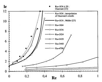
FIG. 10. Characteristic growth length over which the vertical velocity envelope of the transversal rolls,  $W_{\rm max}(x)$ , increases from the inlet to half its value of saturation ( $W_s/2$ ), as a function of Re; at Ra=1836, comparison with Ouazzani's experiment<sup>23</sup> and with a result obtained from the amplitude equation theory by Müller.<sup>23</sup>
