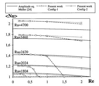
FIG. 13. Space and time average Nusselt number as a function of Re and Ra; comparison of the numerical solutions obtained on config-1 and config-2 with the linear stability result obtained by Müller.<sup>24</sup>
