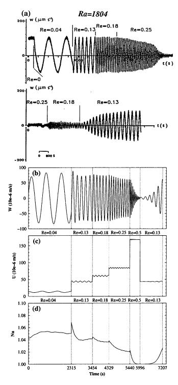
FIG. 7. The same as Fig. 4 for Ra=1804 and Re=0.04, 0.13, 0.18, and 0.25 (plus Re=0.5 for the numerical simulation); (a) for the experiment,  $^{14,16}$  transition to the Poiseuille flow at Re=0.25; (b),(c),(d) for the 2-D numerical simulation, transition to the Poiseuille flow at Re=0.5.
