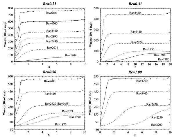
FIG. 9. For fixed Re and several Ra, stationary envelopes representing the space evolution of the maximum vertical velocity component along the axis of the channel, from the inlet to the outlet of config-1 domain; for Re=0.21, 0.5, and 1, A = L/h = 10; for Re=0.31, A = 20.
