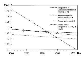
FIG. 16. Ratio of the transversal roll velocity, Vr, to the average velocity of the flow,  $U^{\circ}$ , as a function of Ra and for Pr=6.4; comparison of the numerical solutions obtained on config-1 and config-3 with the experimental results of Ouazzani *et al.*<sup>14,16</sup> and with Müller's theoretical result<sup>24</sup> (the limit of validity of this theory, Ra $\approx$ 2500, is indicated by a vertical line). All the curves are independent of Re.
