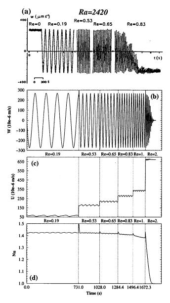
FIG. 5. The same as Fig. 4 for Ra=2420 and Re=0.19, 0.53, 0.65, and 0.83 (plus Re=1 and Re=2 for the numerical simulation); (a) for the experiments,  $^{14,16}$  transition to longitudinal rolls at Re=0.83; (b),(c),(d) for the 2-D numerical simulations, transition to the Poiseuille flow at Re=2.
