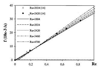
FIG. 14. Transversal roll frequency, computed on config-1, as a function of Re and Ra and for Pr=6.4; comparison with Ouazzani's experiment<sup>14</sup> at Ra=2024 and 2420.
