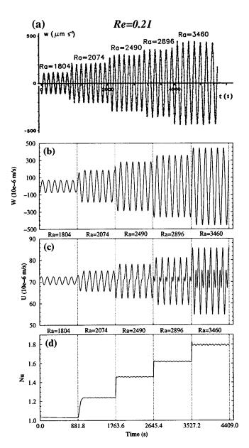
FIG. 4. Time evolution in the transversal roll phase, of the vertical [W(t)] and horizontal [U(t)] velocity components and of the space average Nusselt number [Nu(t)] for Re=0.21, Ra=1804, 2074, 2490, 2896, and 3460, and for Pr=6.4; (a) W(t) at (x,z)=(15.7, 0.5) from the experiments of Ouazzani et al.; <sup>14,16</sup> (b),(c),(d), respectively, W(t), U(t), and Nu(t) at (x,z)=(7.5, 0.5) for the present numerical work (config-1).
