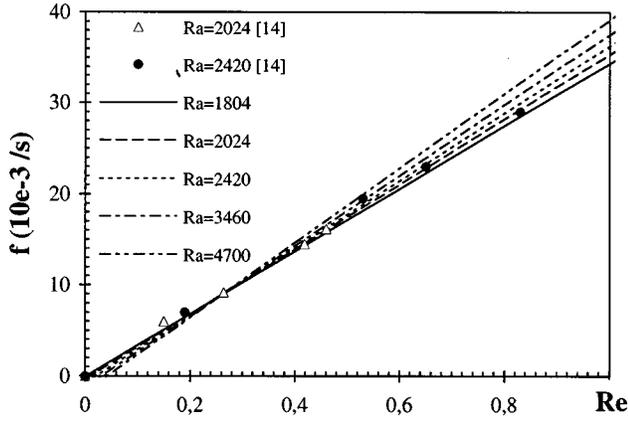
FIG. 14. Transversal roll frequency, computed on config-1, as a function of  $Re$  and  $Ra$  and for  $Pr=6.4$ ; comparison with Ouazzani's experiment<sup>14</sup> at  $Ra=2024$  and  $2420$ .
