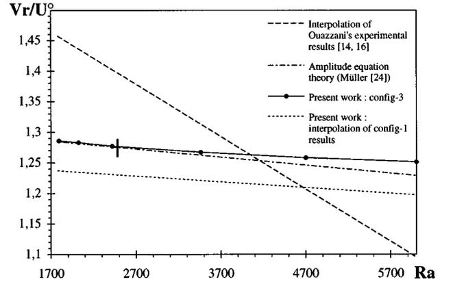
FIG. 16. Ratio of the transversal roll velocity,  $Vr$ , to the average velocity of the flow,  $U^\circ$ , as a function of  $Ra$  and for  $Pr=6.4$ ; comparison of the numerical solutions obtained on config-1 and config-3 with the experimental results of Ouazzani *et al.*<sup>14,16</sup> and with Müller's theoretical result<sup>24</sup> (the limit of validity of this theory,  $Ra \approx 2500$ , is indicated by a vertical line). All the curves are independent of  $Re$ .
