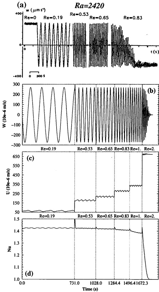
FIG. 5. The same as Fig. 4 for  $Ra=2420$  and  $Re=0.19, 0.53, 0.65,$  and  $0.83$  (plus  $Re=1$  and  $Re=2$  for the numerical simulation); (a) for the experiments,<sup>14,16</sup> transition to longitudinal rolls at  $Re=0.83$ ; (b),(c),(d) for the 2-D numerical simulations, transition to the Poiseuille flow at  $Re=2$ .
