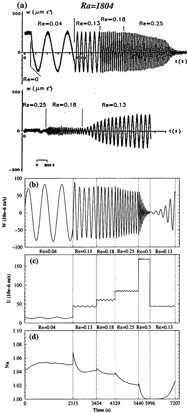
FIG. 7. The same as Fig. 4 for  $Ra=1804$  and  $Re=0.04, 0.13, 0.18,$  and  $0.25$  (plus  $Re=0.5$  for the numerical simulation); (a) for the experiment,<sup>14,16</sup> transition to the Poiseuille flow at  $Re=0.25$ ; (b),(c),(d) for the 2-D numerical simulation, transition to the Poiseuille flow at  $Re=0.5$ .
