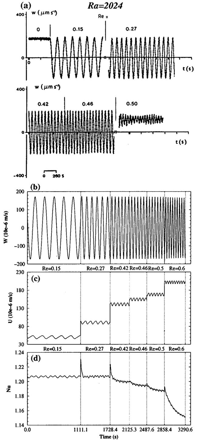
FIG. 6. The same as Fig. 4 for  $Ra=2024$  and  $Re=0.15, 0.27, 0.42, 0.46,$  and  $0.5$  (plus  $Re=0.6$  for the numerical simulation); (a) for the experiment,<sup>14</sup> transition to “intermittent pattern” at  $Re=0.5$ ; (b),(c),(d) for the 2-D numerical simulation, persistence of the Poiseuille flow until  $Re=0.6$ .
