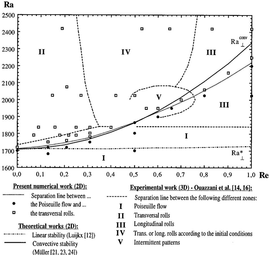
FIG. 12. Stability diagram of the different configurations encountered in the PBF with  $Pr=6.4$ . The numerical results of the present work are obtained with config-1; other already published results are superimposed to the numerical solution.
