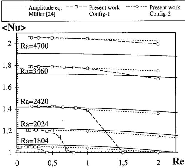
FIG. 13. Space and time average Nusselt number as a function of  $Re$  and  $Ra$ ; comparison of the numerical solutions obtained on config-1 and config-2 with the linear stability result obtained by Müller.<sup>24</sup>
