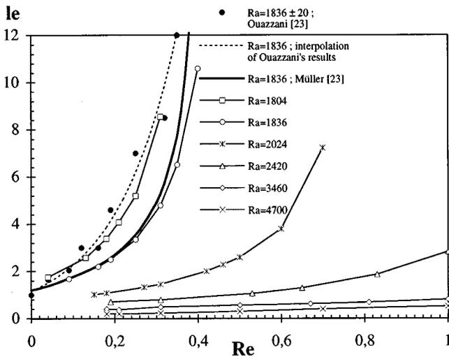
FIG. 10. Characteristic growth length over which the vertical velocity envelope of the transversal rolls,  $W_{\max}(x)$ , increases from the inlet to half its value of saturation ( $W_s/2$ ), as a function of  $Re$ ; at  $Ra=1836$ , comparison with Ouazzani's experiment<sup>23</sup> and with a result obtained from the amplitude equation theory by Müller.<sup>23</sup>
