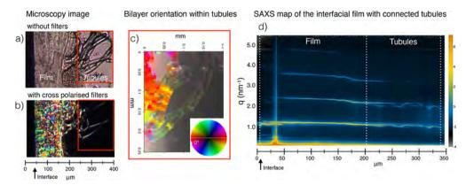
**Figure 6.** Microscopy images without (a) and with (b) crossed polarizers, showing tubule formation at the film growth front. (c) Orientation map from 2D SAXS patterns show that lamellar domains are weakly oriented along curls in the tubules. (d) SAXS map showing that tubules are made from lamellae directly connected to the film and with similar spacing as within the inner part of the film.
