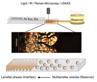
**Figure 1.** Schematic view of the millifluidic setup, which consists of a rectangular capillary connected on one end to a reservoir of the Curosurf vesicular dispersion and exposed on its other end to an air flux of controlled relative humidity (RH). Water evaporation leads to the buildup of a multilamellar film through multilamellar vesicle fusion, which is birefringent under crossed polarizer observation.
