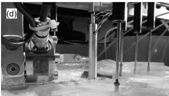
Figure 3: Experimental model: (a) cross section in the load plane, (b) aerial view of the basket, (c) perspective of valve system and soil container, (d) detail of the loading system and LVDT.
