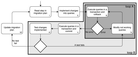
Fig. 2: Process formalized from the database architect actions
