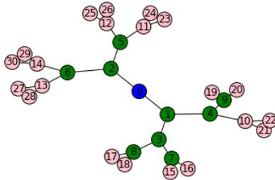
Figure 1: Example of a radial network. The root node at the interface of the distribution and transmission networks, can trade energy with any other node in the distribution network. In the distribution network, prosumer nodes organize in local energy communities, trading energy with neighbors inside their local community.
