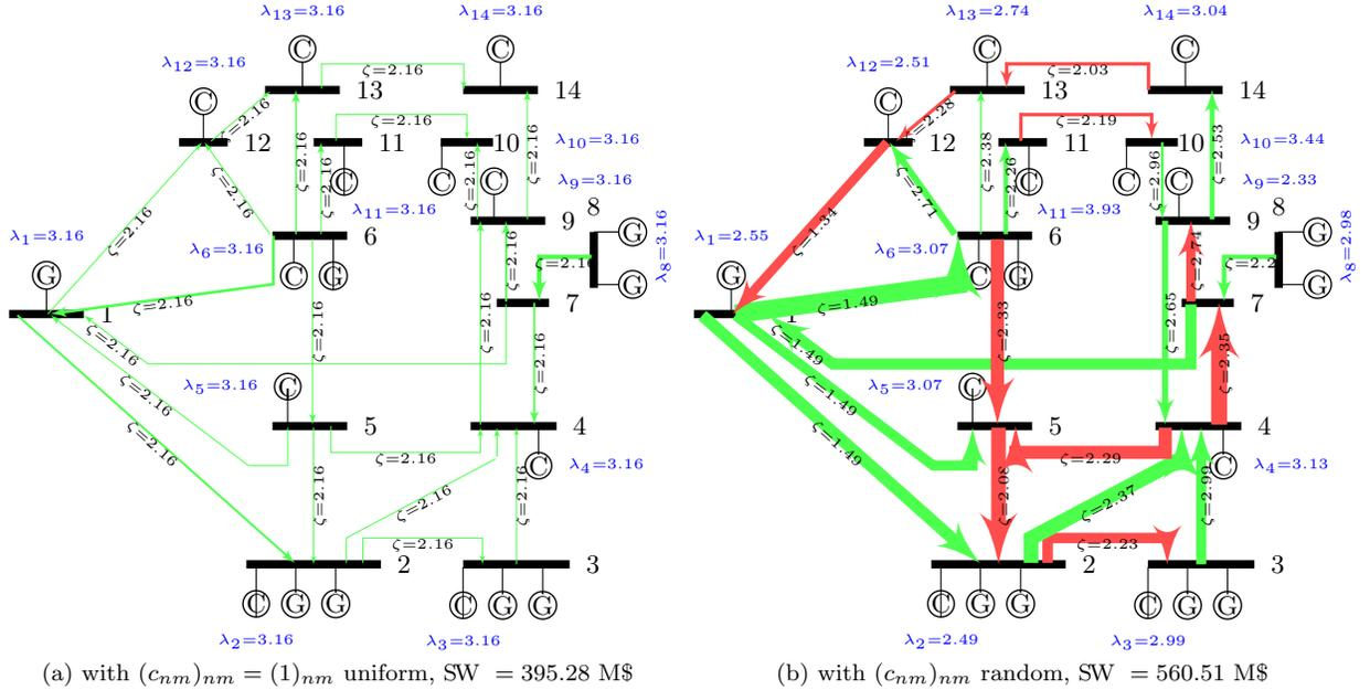
Figure 6: Trades [\$/MWh] at the VNE of the IEEE 14-bus network with homogeneous differentiation prices (left) and heterogeneous differentiation prices (right). *With heterogeneous prices, the quantities traded are larger, and some links become congested. In the heterogeneous case, marginal trade prices  $(\zeta_{nm})_{n,m}$  are all equal. In the case of heterogeneous prices  $(c_{nm})_{nm}$ , marginal prices  $(\zeta_{nm})_{n,m}$  are also heterogeneous.*
