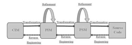
Figure 3. The MDA model refinement and transformation process.
