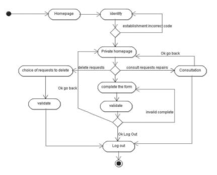
Figure 11. An activity diagram of the head of the main maintenance of the component parts of passengers and baggage railcars.
