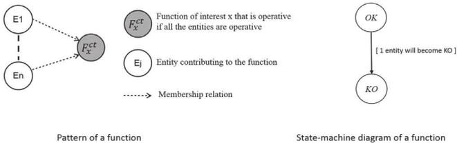
Fig. 6. Pattern and state-machine diagram of a function.
