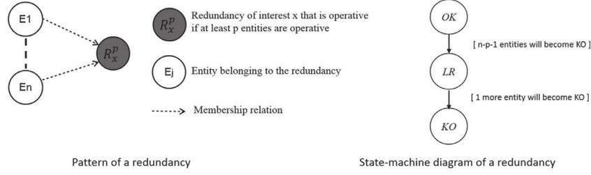
Fig. 5. Pattern and state-machine diagram of a redundancy.
