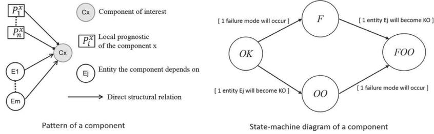
Fig. 4. Pattern and state-machine diagram of a component.
