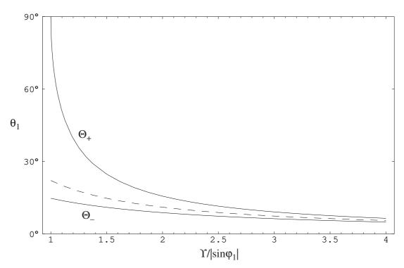
Figure 6. Equation of the caustics for an oscillating source in uniform horizontal motion; (---) exact equation (4.5), (---) asymptotic equation (4.6) (from [35]).
