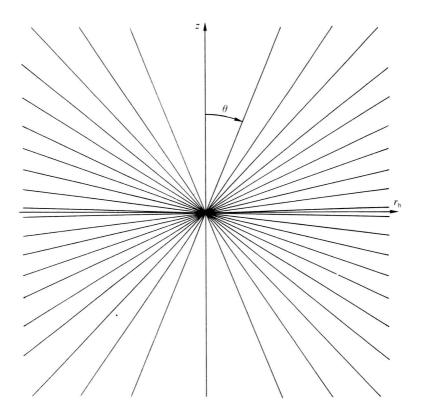
FIGURE 3. Surfaces of constant phase  $\Phi = \pi/4 + n\pi$  for a point impulsive source, for  $Nt = 10\pi$  (from [25]).
