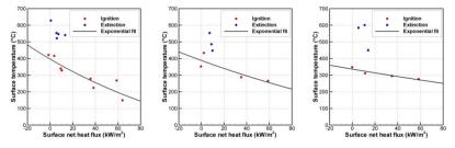
Fig. 3.  $T_{ig}$  vs.  $\dot{q}_{net}$  correlation – from left to right: CLT, birch plywood and okoume plywood.
