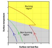
Fig. 4: Trajectory examples in heat transfer space phase
