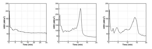
Fig. 2. HRR measurements - from left to right: CLT, birch plywood and okoume plywood.
