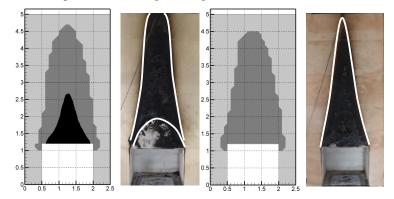
Fig. 5: Facades after burning - From left to right: Birch simulation and test, okoume simulation and test
