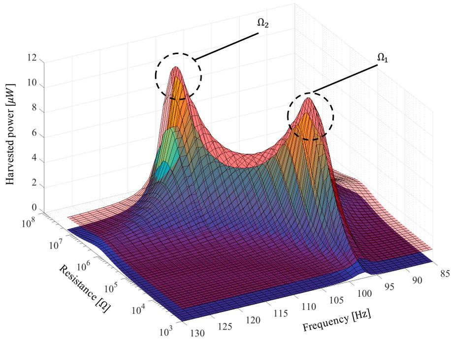
**Fig. 12.** Comparison between experimental (colored surface) and theoretical (transparent surface) harvested power on a resistive load in the  $(R, f)$  plane. The theoretical surface has been shifted of  $1\mu\text{W}$  in order to clarify the figure.
