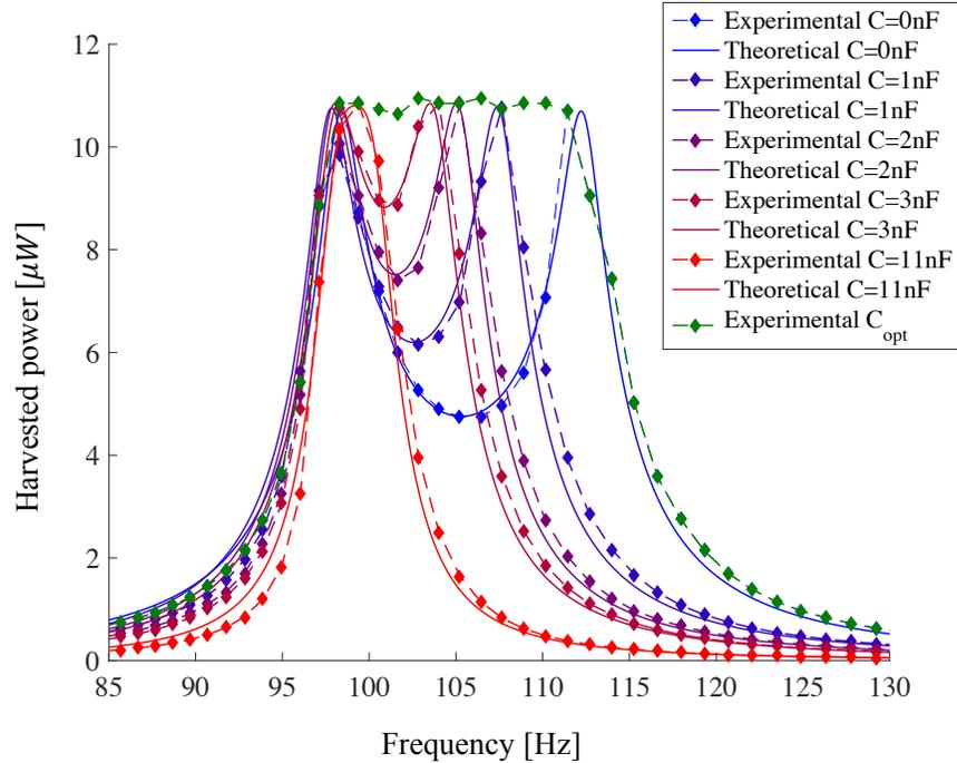
**Fig. 17.** Experimental (dots and dashed lines) and theoretical (straight lines) power frequency responses of our piezoelectric harvester with optimized resistive loads and various capacitive loads.
