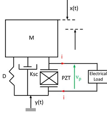
**Fig. 2.** Generic mechanical-to-electrical conversion model
