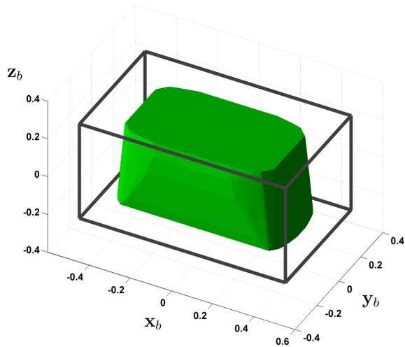
Fig. 10. Larger WFW, covering the 65.98% of the desired workspace, computed with respect to the design variables  $\tau_M = 1.5 \text{ Nm}$ ,  $\omega_M = 200 \text{ rpm}$ ,  $\phi_w = 50 \text{ mm}$ ,  $\rho_R = 5$ .
