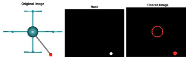
**Figure 2. Resulting images after applying the algorithm.**
