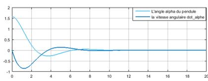
**Figure 3. Simulation result for the angle  $\alpha$  and its velocity of the Spherical Inverted Pendulum**
