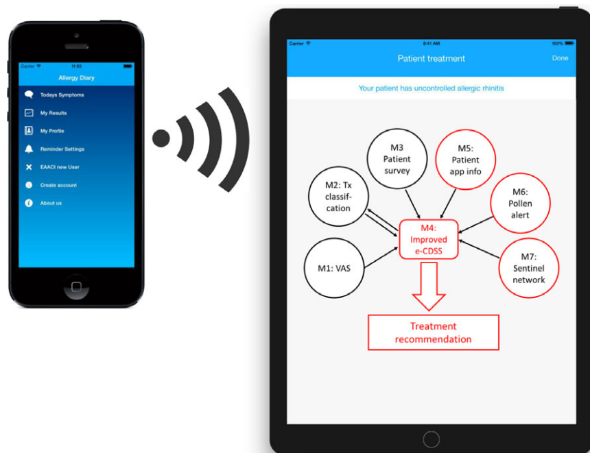
FIGURE 4 Schematic representation of architecture of an improved e-CDSS. M, module; Tx, treatment; e-CDSS, electronic clinical decision support system
