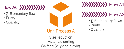
Fig. 5 Modelling of a recycling pathway step with a unit process and its related flows
