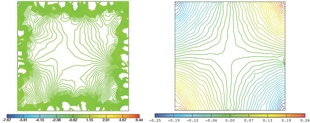
Fig. 9. Computed pressure without (left panel) and with (right panel) harmonic functions in the vorticity–velocity–pressure scheme, extrema:  $-7.67$  to  $6.44$  (left) and  $-0.25$  to  $0.26$  (right).
