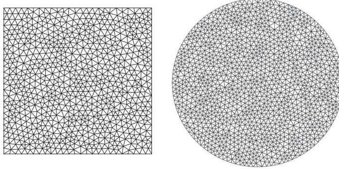
FIG. 2. Two unstructured meshes obtained by EMC2.
