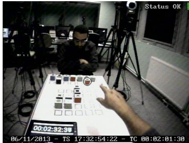
Figure 2: ego-centric view as seen from the instructor and extracted from the cube game experiment. The current fixation point of the right eye – monitored by a Pertech® head-mounted eyetracker – is cued by a back circle (here surrounding the red cube pointed by the hand of the instructor). Time stamps are used to synchronize multimodal streams.
