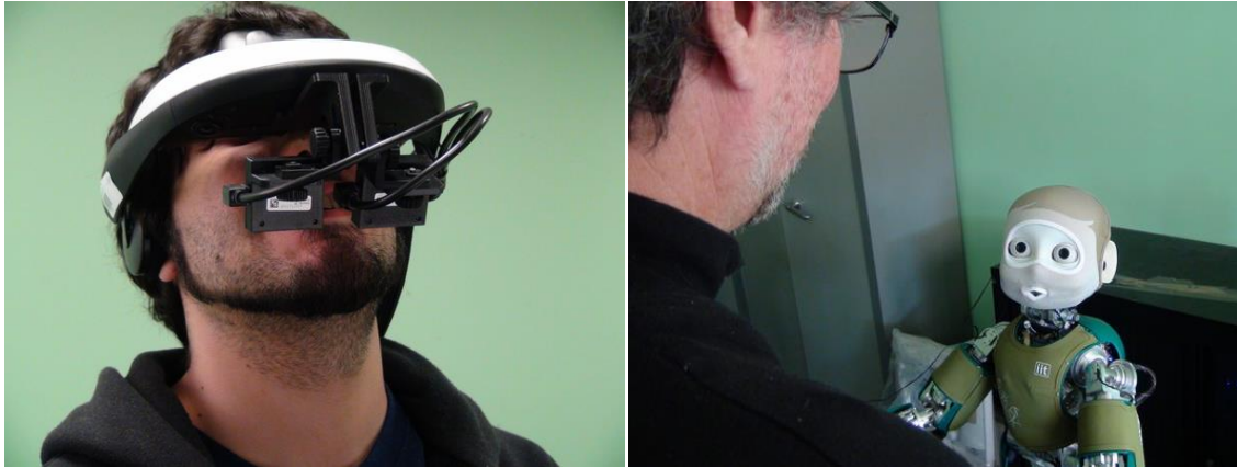
Figure 6. Beaming the GIPSA-Lab iCub: the human tutor (left) monitors the head and eyes of the iCub robot (right) while perceiving (viewing and listening) the remote scene via a head mounted display that plays back the audiovisual streams captured by the cameras and microphones embedded into its eyes and ears. This cognitive gift artificially provides the robot with situated social skills.
