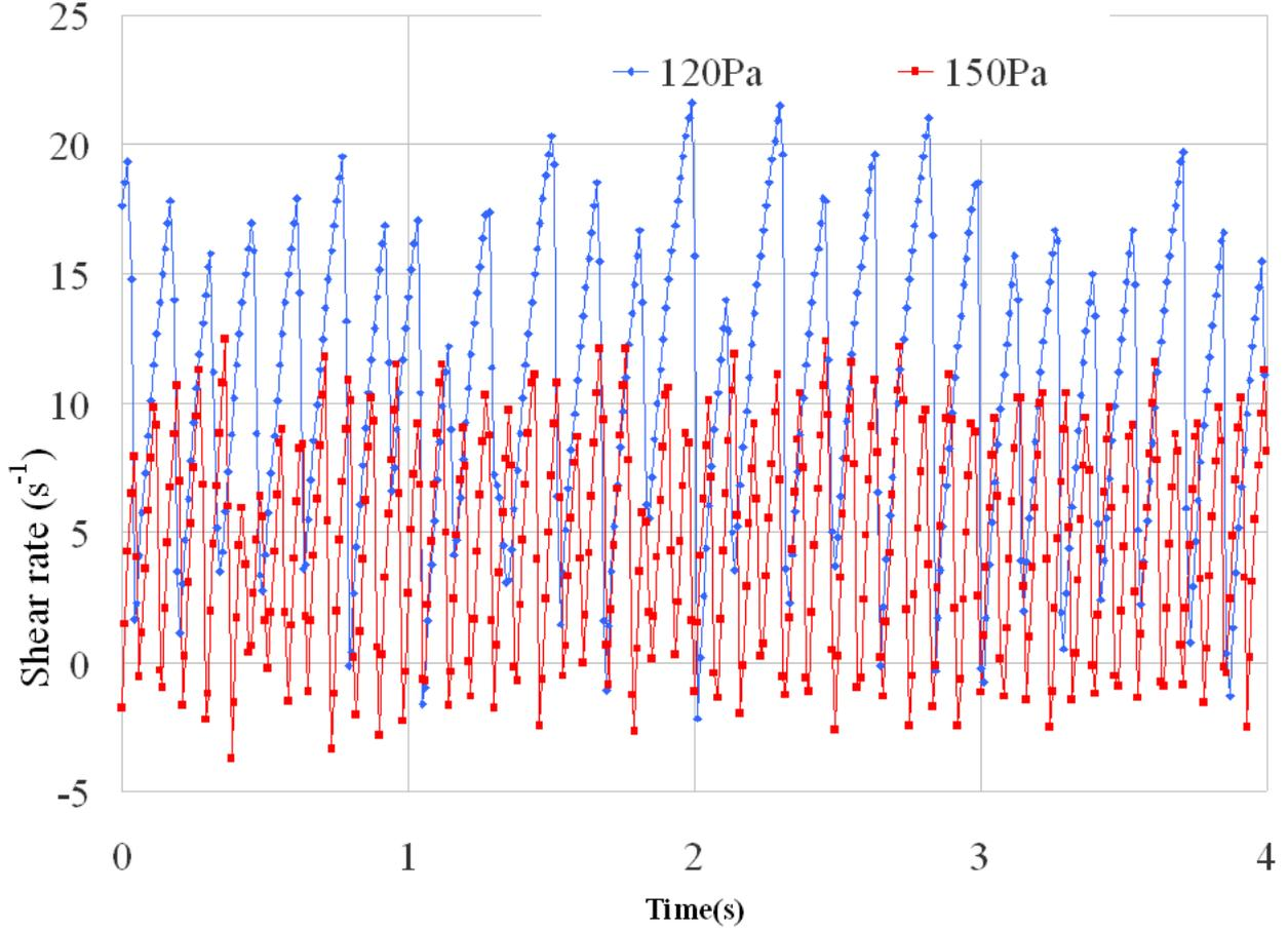
Fig.9 Shear rate versus time for a constant applied stress of 120 Pa and then 150Pa. Carboxy iron suspension in water at  $\Phi=0.62$  with 0.2% weight of PPP44
