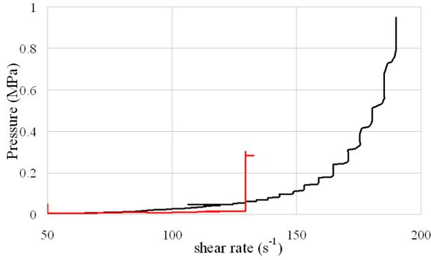
Fig.(14a) Pressure versus shear rate in a capillary rheometer. Suspension of iron  $\Phi=64\%$ . Red curve :slow increase of shear rate (see Fig 13b). Black curve:fast increase ( $60\text{s}^{-1}/\text{mn}$ )
