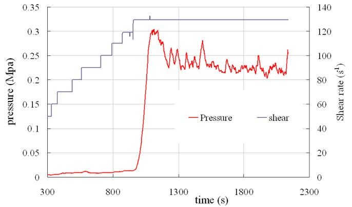
Fig. (14b) : Evolution of shear rate (blue curve) and of the pressure (red curve) with time. It corresponds to the red curve of the left figure.
