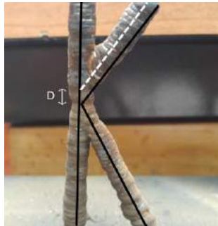
Figure 7: Example of a difference between the desired geometry (in full black lines) and the deposited geometry after the intersection (white dotted line is the neutral axis of deposition).
