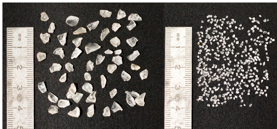
Figure 2. PMMA particles used in the S3 (left, d_p = 3 mm) and S1 (right, d_p = 1 mm) experiments. PMMA = polymethyl methacrylate.
