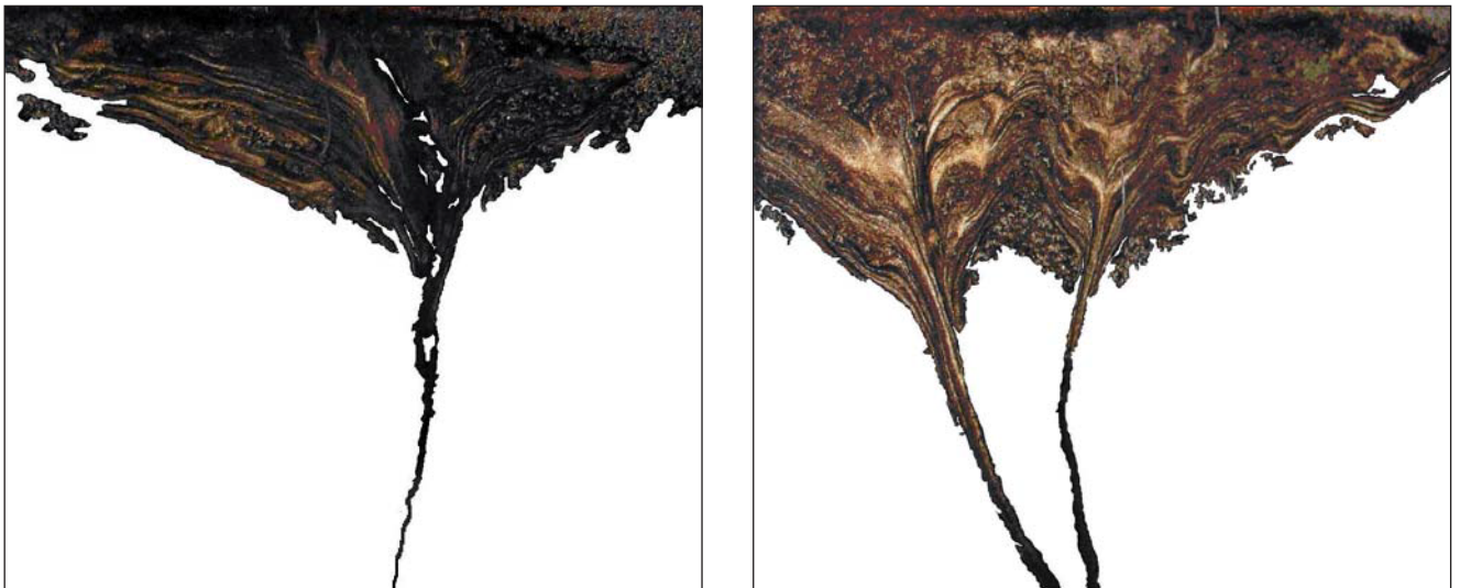
Figure 11 Presentation of spreading stage of solvent chamber without MMTs (left) and using MMTs (right) after 9 h.
