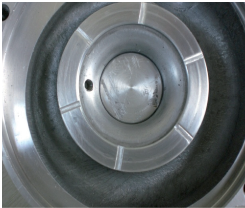
Figure 8 Tested grooves on pinched diffuser (GRP).
