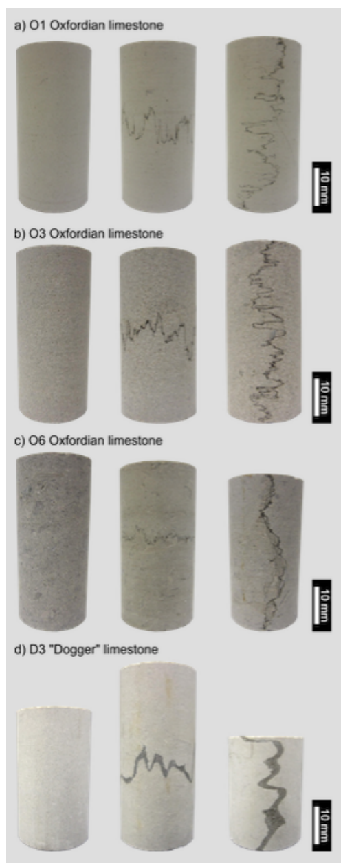
514 Figure 6. Photographs of the cylindrical samples prepared for laboratory measurements. Three 515 representative samples are shown for each lithology: an intact sample (on the left), a sample with a 516 stylolite perpendicular to flow (in the middle), and a sample with a stylolite parallel to flow (on the 517 right). (a) Sample O1 – Oxfordian limestone from Bure. (b) Sample O3 – Oxfordian limestone from 518 Bure. (c) Sample O6 – Oxfordian limestone from Bure. (d) Sample D3 – “Dogger” limestone from 519 Bure.
