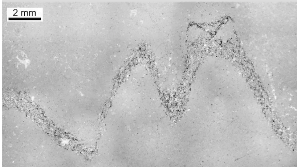
a) D3 "Dogger" limestone - thick stylolite
