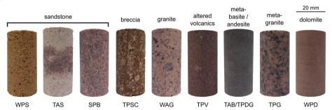
**Fig. 3** Photos of the rock samples prepared for physical property characterisation. *WPS* sandstone from Raon l'Etape, *TAS* sandstone from Waldhambach, *SPB* sandstone from Saint Pierre Bois, *TPSC* breccia from Albersweiler, *WAG* granite from Saint Pierre Bois, *TPV* hydrothermally altered volcanic rock from Albersweiler, *TAB* hydrothermally altered andesite from Waldhambach, *TPDG* metabasite from Albersweiler, *TPG* metagranite from Albersweiler, *WPD* dolomite from Raon l'Etape
