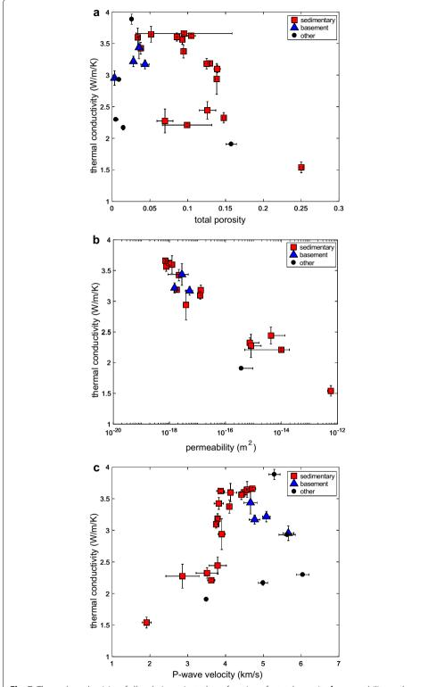
**Fig. 7** Thermal conductivity of all rocks investigated as a function of **a** total porosity, **b** permeability, and **c** P-wave velocity. All rocks are categorised as either sedimentary (red squares), crystalline basement (blue triangles), or other lithologies (black circles); see Table 2. Thermal conductivity, porosity, permeability and P-wave velocities shown are the mean values for each rock type; error bars indicate the standard deviation of each mean value
