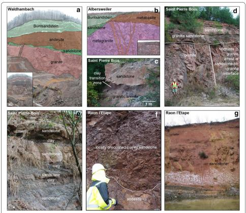
**Fig. 2** Photos of the field locations from which the rock samples were taken. The dominant lithologies at each site are indicated. **a** Waldhambach, Germany. **b** Albersweiler, Germany. **c** Saint Pierre Bois, France. **d** Saint Pierre Bois, France. Note the fractures present in the granite become arrested at the sandstone–granite interface. **e** Saint Pierre Bois, France. Note the alternating sandstone and clay units. **f** Raon l'Etape, France. **g** Raon l'Etape, France
