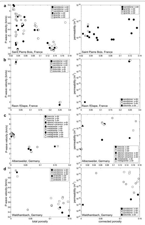
**Fig. 6** P-wave velocity as a function of total porosity and permeability as a function of connected porosity for all rocks, organised by sample location. **a** Saint Pierre Bois. **b** Raon l'Etape. **c** Albersweiler. **d** Waldhambach
