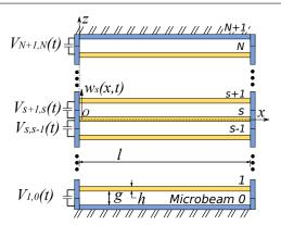
Fig. 1 Model of the clamped-clamped microbeam array.
