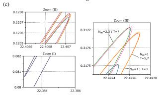
**Fig. 3** Nonlinear forced response curves of a two-beam array without added mass by HBM+ANM method. Responses with third (blue), fifth (red) and seventh (orange) order Taylor series and  $N_m = 1$  mode; responses with seventh-order Taylor series with  $N_m = 2$  (pink) or  $N_m = 3$  (green) modes. Dark and light blue colors indicate stable and unstable solutions respectively. (a): Beam #1, (b): Beam #2, (c): zoom of (I), (III), (III).
