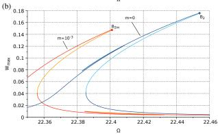
**Fig. 10** Response with  $V_{dc_{32}} = V_{ac_{32}} = 0.575V$  and other voltages as in Table 1, without mass (dark/light blue) and with  $m = 10^{-3}$  (red/orange). (a): Beam #1, (b): Beam #2.
