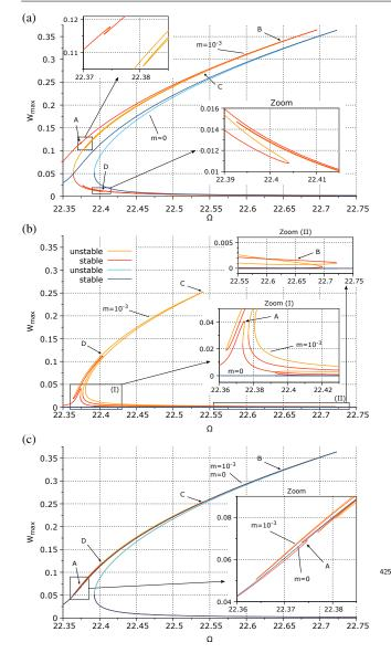
Fig. 12 Design #2: response with a mass  $m = 10^{-3}$  added on the first beam (red/orange) and without added mass (dark/light blue). (a): Beam #1, (b): Beam #2, (c): Beam #3. Without added mass, the second-beam amplitude is nil.
