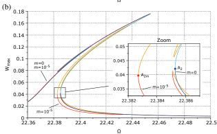
**Fig. 9** Response with  $V_{dc_{32}} = V_{ac_{32}} = 0.575V$  and other voltages as in Table 1, without mass (dark/light blue) and with  $m = 10^{-5}$  (red/orange). (a): Beam #1, (b): Beam #2.
