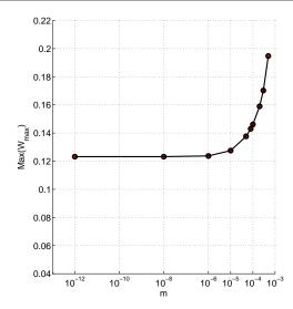
Fig. 18 Design #4. Maximum of amplitude  $Max(W_{max})$  with respect to added mass m for Beam #2.
