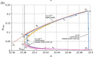
Fig. 8 Design #1. Responses determined by time integration method without added mass (blue curves  $J_1 - i_1 - ji_1 - C_1 - J_1$  and  $J_2 - i_2 - J_1$  $ji_2 - g_2 - d_2 - jd_2 - J_2$ ) and with added mass  $m = 10^{-4}$  (green curves  $J_1 - I_1 - jI_1 - G_1 - H_1 - jH_1 - J_1$  and  $J_2 - I_2 - jI_2 - G_2 - J_2$ ); responses determined by HBM+ANM with added mass  $m = 10^{-4}$  (red: stable branches, orange: unstable branches). (a): Beam #1, (b): Beam #2.
