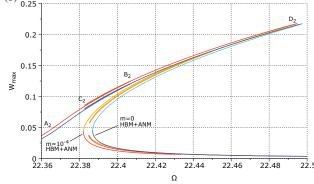
Fig. 6 Design #1. Responses determined by the HBM+ANM method with an added mass  $m = 10^{-4}$  (red: stable branches, orange: unstable branches) and without added mass (dark blue: stable branches, light blue: unstable branches). (a): Beam #1, (b): Beam #2.
