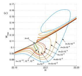
**Fig. 17** Design #4. Responses with  $N_m = 1$  mode and seventh order Taylor series, without added mass (black), with  $m = 10^{-12}$  (green),  $m = 10^{-6}$  (magenta),  $m = 10^{-4}$  (red),  $m = 5 \times 10^{-4}$  (blue) added on the first beam. (a): Beam #1, (b): Beam #2, (c): Beam #3.
