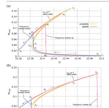
Fig. 7 Design #1. Responses with added mass  $m = 10^{-4}$ . Comparison between HBM+ANM (red: stable branches, orange: unstable branches) and time integration method with a frequency sweep-up (pink curves) and a frequency sweep-down (blue curves). (a): Beam #1, (b): Beam #2..
