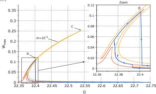
**Fig. 14** Design #2. Response of Beam #2 with  $m=10^{-3}$  added on Beam #1. (a): HBM+ANM (red/orange curve), time integration with a sweep-up (pink curve) and a sweep-down (blue curve); (b): HBM+ANM (red/orange curve), time integration method combining a frequency sweep-down then sweep-up (blue curve).
