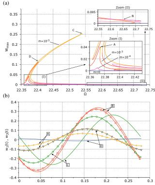
Fig. 13 Design #2: (a): response of Beam #2 without (blue curve) and with  $m = 10^{-4}$  (pink curve) or  $m = 10^{-3}$  (red/orange curve) added on Beam #1. (b): displacement of Beam #1 (solid line) and Beam #3 (dotted line) at points A (yellow curves), B (red curves), C (green curves) and D (blue curves) with  $m = 10^{-3}$ .
