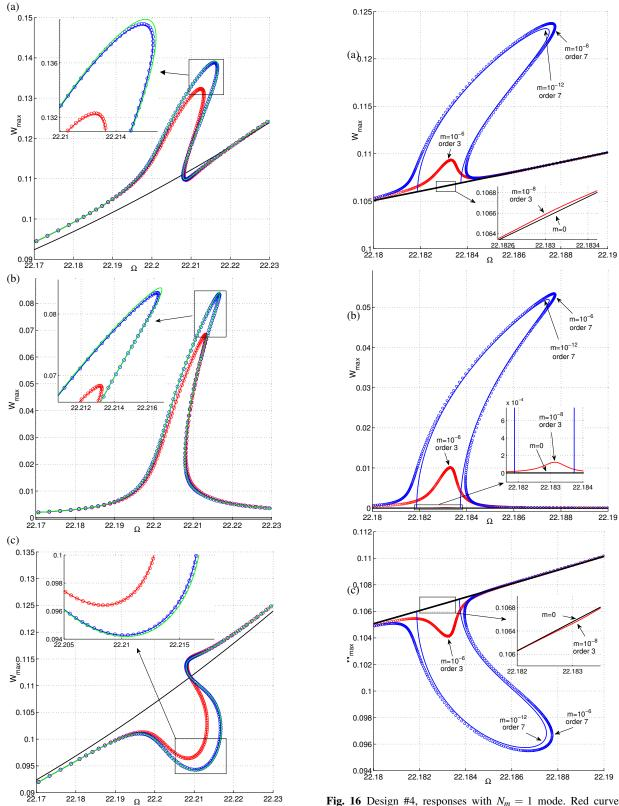
**Fig. 15** Design #3, responses with an added mass  $m = 10^{-4}$  on the first beam determined by using third (red), fifth (blue) and seventh (green) order Taylor series with  $N_m = 1$  (solid line) or  $N_m = 2$  (circle) modes; responses without added mass (black). (a): Beam #1, (b): Beam #2, (c): Beam #3.
