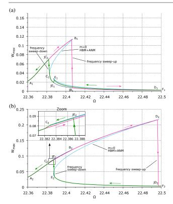
Fig. 5 Design #1. Comparison between HBM+ANM (dark blue: stable branches, light blue: unstable branches) and time integration method with a frequency sweep-up (pink curves) and a frequency sweep-down (green curves). (a): Beam #1, (b): Beam #2.
