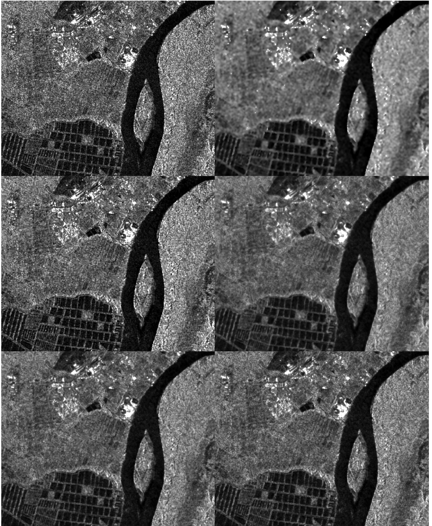
Figure 2. Denoising with the proposed method. Top-left: original amplitude signal. Top-right: Sigma-Lee filtering. Middle-Left: SAR-BM3D. Middle-Right: Pure shrinkage in SVD space (only one singular value retained). Bottom-left: Low-rank transfer with 5 singular values. Bottom-right: Low-rank transfer with 10 singular values.
